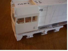
Anti-Climb Sill, Buffer Plate with Kadee coupler #906 and Cow Catcher are now in place.
