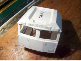
Blocks for housings for lights and number boards were fitted and glued into recesses milled earlier.
