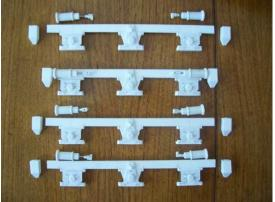
Sandboxes and Air Cylinders fabricated and ready to fit, now for the Springs.
