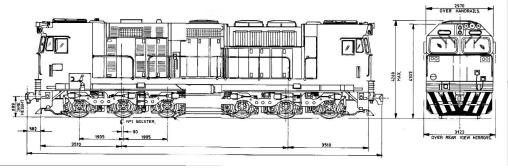
Drawing of the BTR version of 2800 Class loco as "<u>foreshortened</u>" for the minimum 2.4m diameter curves on BTR track and as used to make the model.
