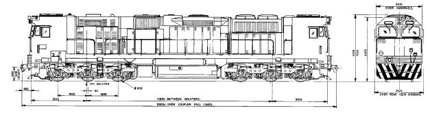
The drawing above is of a VLine N Class that is similar to and indicative of the real Queensland Railways 2800 Class Locomotive [nominally 124 tonnes]. Geof has yet to locate a QR drawing.
